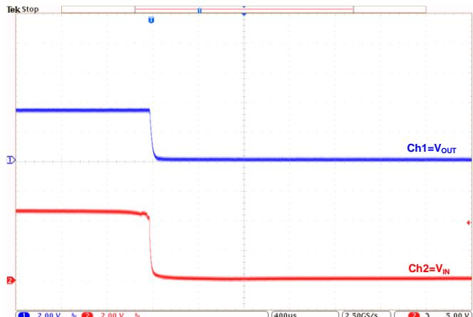
Power-Down at  $V_{OUT}=3.3V$ :
