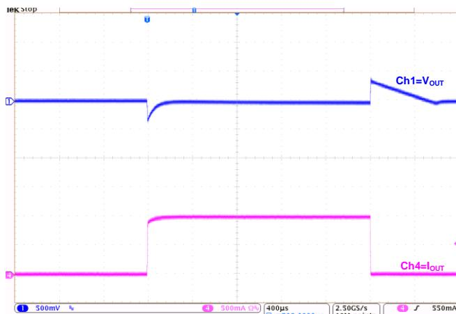
Load Transient at  $V_{OUT}=3.3V$
