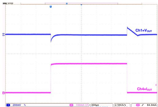
Load Transient at  $V_{OUT}=3.3V$
