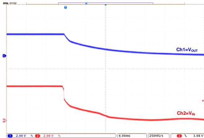
Power-Down at  $V_{OUT}=3.3V$ :
