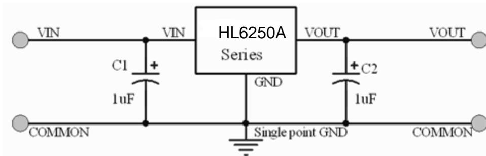
Note1: Input capacitor  $C_{IN}=1\mu F$ .
