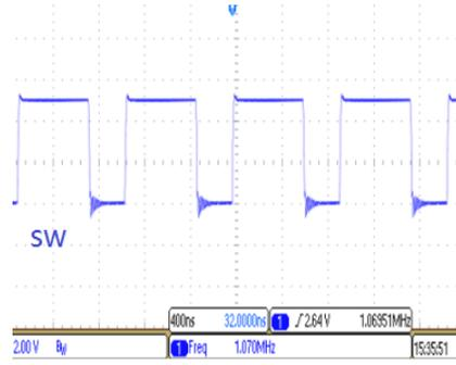
Fig 4 SW Waveform
