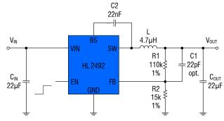
Figure 1. Basic Application Circuit
